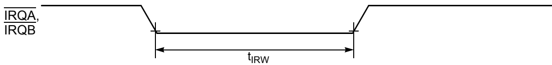
Figure 10-6 External Interrupt Timing (Negative Edge-Sensitive)
