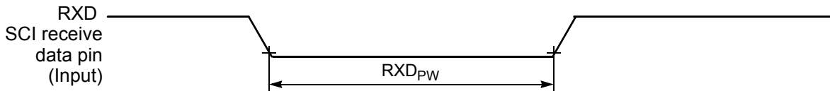
Figure 10-16 RXD Pulse Width
