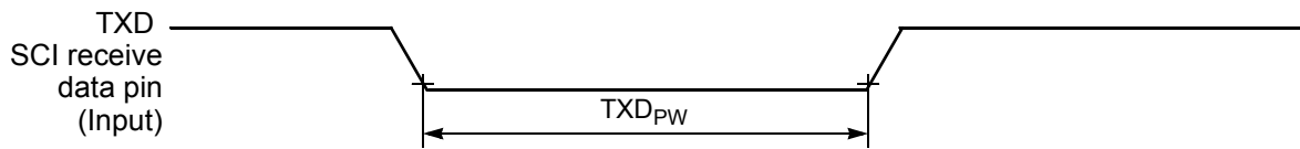
Figure 10-17 TXD Pulse Width
