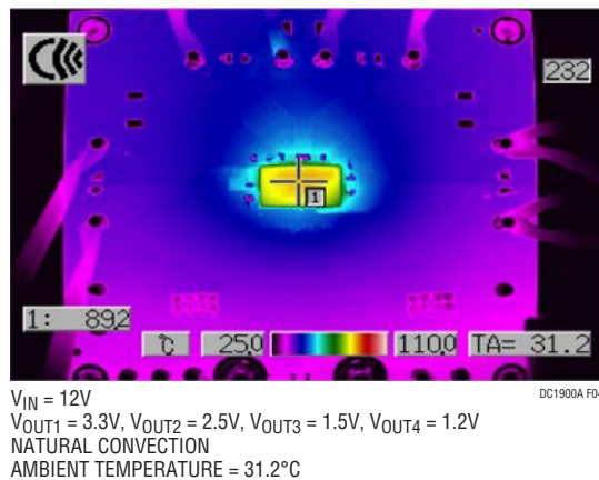
Figure 4. Measured Thermal Capture with All Phases at Full Load (4A)
