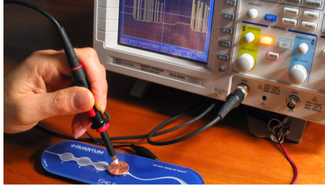
Figure 2-1. Measuring the Charge-transfer Pulses
