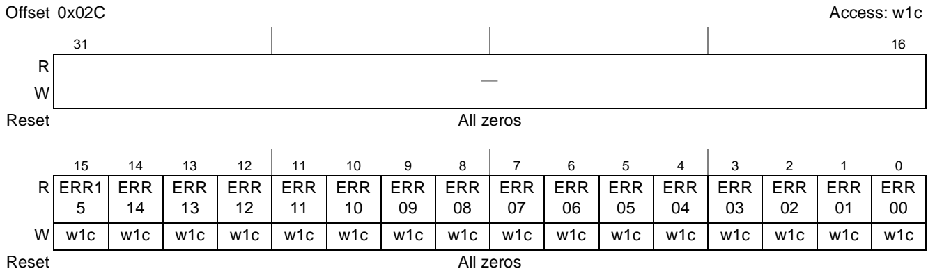
Figure 12-12. DMA Error Register (DMAERR)
