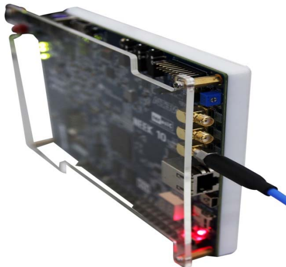
Figure 5-9 Probe DAC SMA OUT from the oscilloscope
