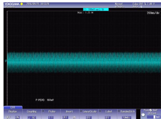
(b) 230V (measured value=187mV)
