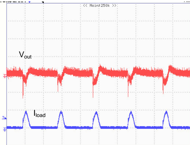
Figure 54 – +28 V Sine Load, 115 VAC, 444 mA Load. Upper: Output Voltage, 20 mV / div. Lower: Load Current, 500 mA / div & 50 ms / div.
