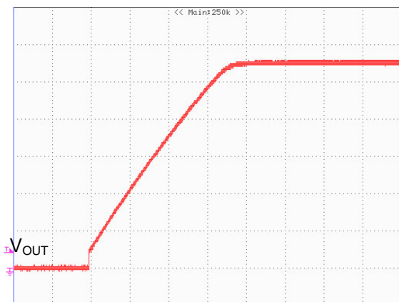
Figure 28 – Start-up Profile +28 V Output, 90VAC Full Load, 5 V, 50 ms / div.
