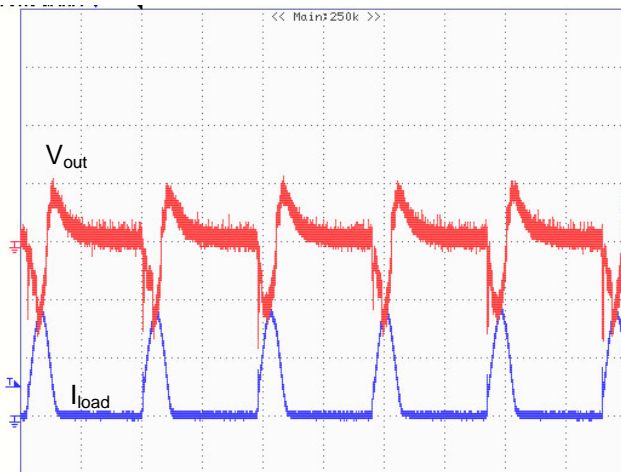
Figure 55 – +28 V Sine Load, 115 VAC, 889 mA Load. Upper: Output Voltage, 20 mV / div. Lower: Load Current, 500 mA / div & 50 ms / div.
