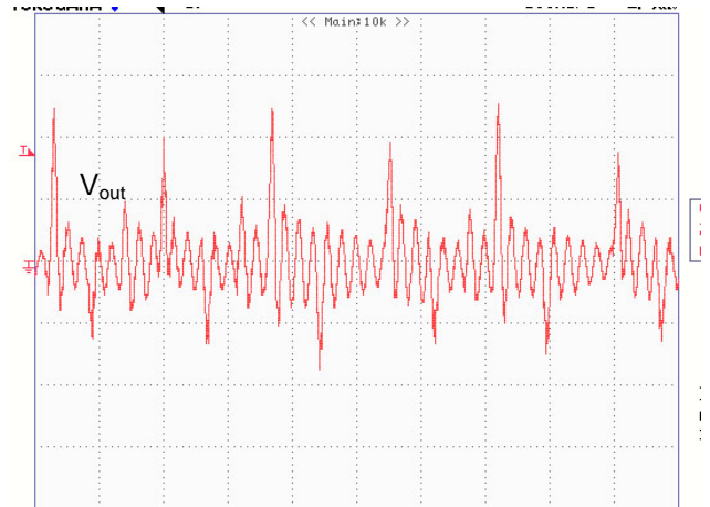
Figure 53 – +12 V Ripple, 90 VAC, 333 mA Load. (3.57 A load on Main) 2 \mu s, 20 mV / div.
