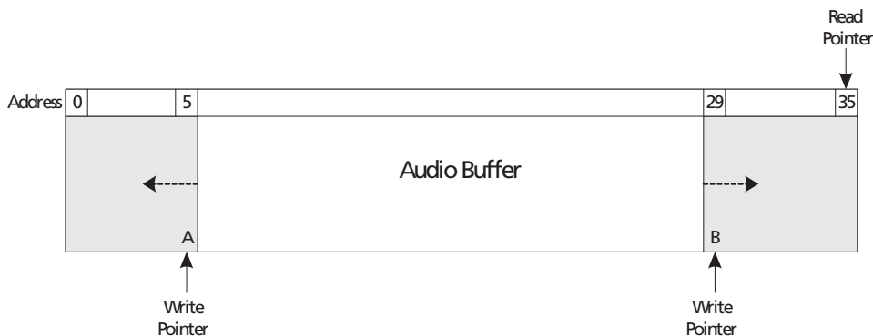
Figure 4-44: Audio Buffer Pointer Boundary Checking
