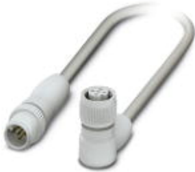
Sensor/Actuator cable, 5-position, PP-EPDM halogen-free, Gray RAL 7035, Plug straight M12, A-coded, on Socket angled M12, A-coded, Cable length: 0.3 m, Hygienic design, with plastic knurl
