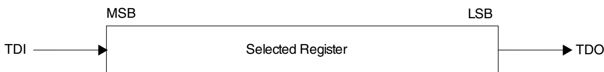
Figure 49-3. Shifting data through a register
