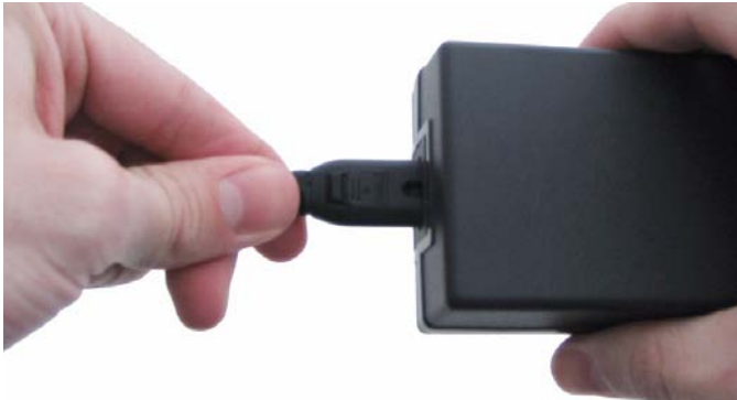
Figure 3.1 – Connect Power Supply and Adapter
