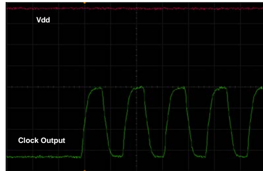
Figure 18. Startup Waveform vs. Vdd (Zoomed-in View of Figure 17)
