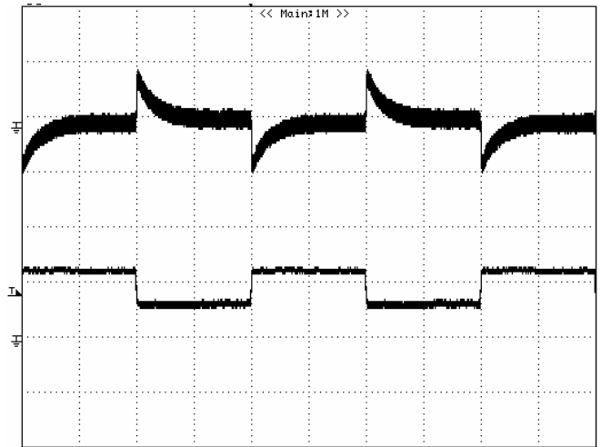
Figure 7: Output voltage response to step-change in load current (50%-25%-50% of I_o , max; di/dt = 2.5A/\mu s ). Load cap: 10\mu F , tantalum capacitor and 1\mu F ceramic capacitor. Top Trace: V_{out} (200mV/div, 500us/div), Bottom Trace: I_{out} (2A/div). Scope measurement should be made using a BNC cable (length shorter than 20 inches). Position the load between 51 mm to 76 mm (2 inches to 3 inches) from the module
