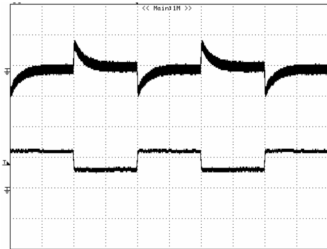
Figure 6: Output voltage response to step-change in load current (50%-25%-50% of I_o , max; di/dt = 0.1A/\mu s ). Load cap: 10\mu F , tantalum capacitor and 1\mu F ceramic capacitor. Top Trace: V_{out} (200mV/div, 500us/div), Bottom Trace: I_{out} (2A/div). Scope measurement should be made using a BNC cable (length shorter than 20 inches). Position the load between 51 mm to 76 mm (2 inches to 3 inches) from the module
