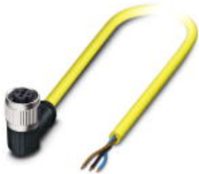
Sensor/Actuator cable, 3-position, TPE, yellow RAL 1021, free cable end, on Socket angled M12 SPEEDCON, A-coded, Cable length: 10 m
