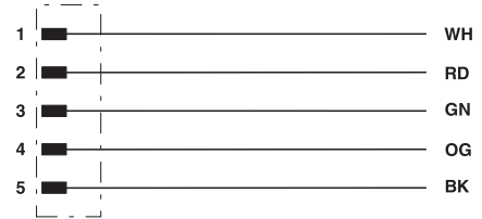
Contact assignment of 7/8" plug
