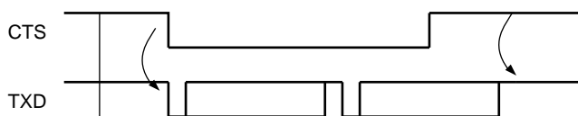
Figure 31-19. Transmitter Behavior when Operating with Hardware Handshaking
