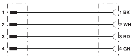
Contact assignment of 7/8" plugs/sockets
