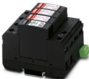
Surge arrester consisting of base element with remote indicator contact and ground connectors, for mounting on NS 35/7.5, nominal voltage: 120 V AC, 3 + 1 circuit
